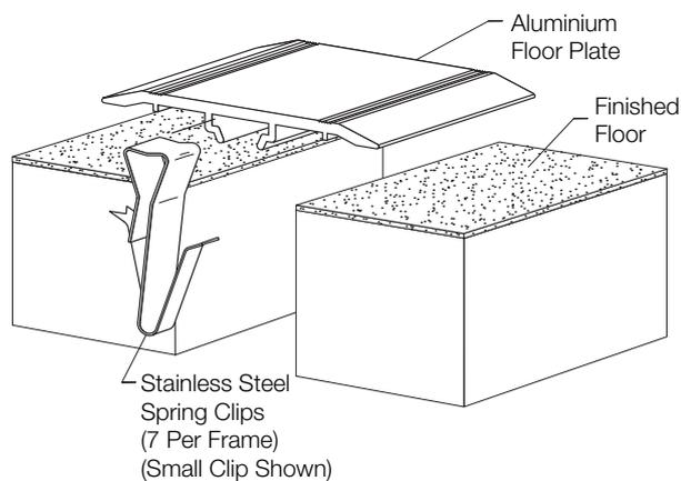
**1.** Install the architectural joint system on a level finished floor or wall surface. This may require adding leveling compound on top of the substrate to provide a smooth mounting surface.
