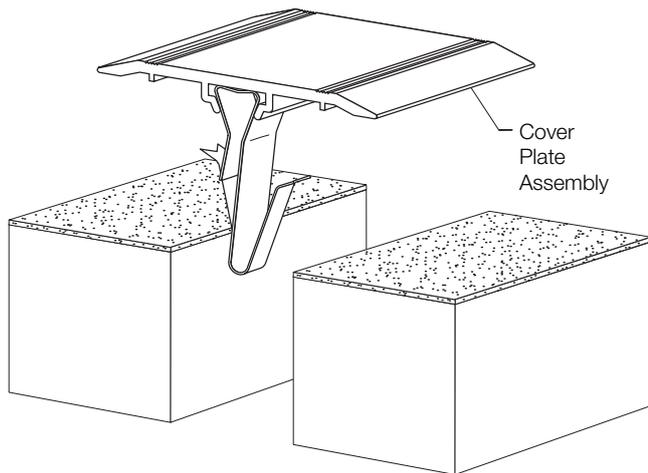
**4.** Firmly squeeze the top of the spring clip and slide down the channel to desired location.
